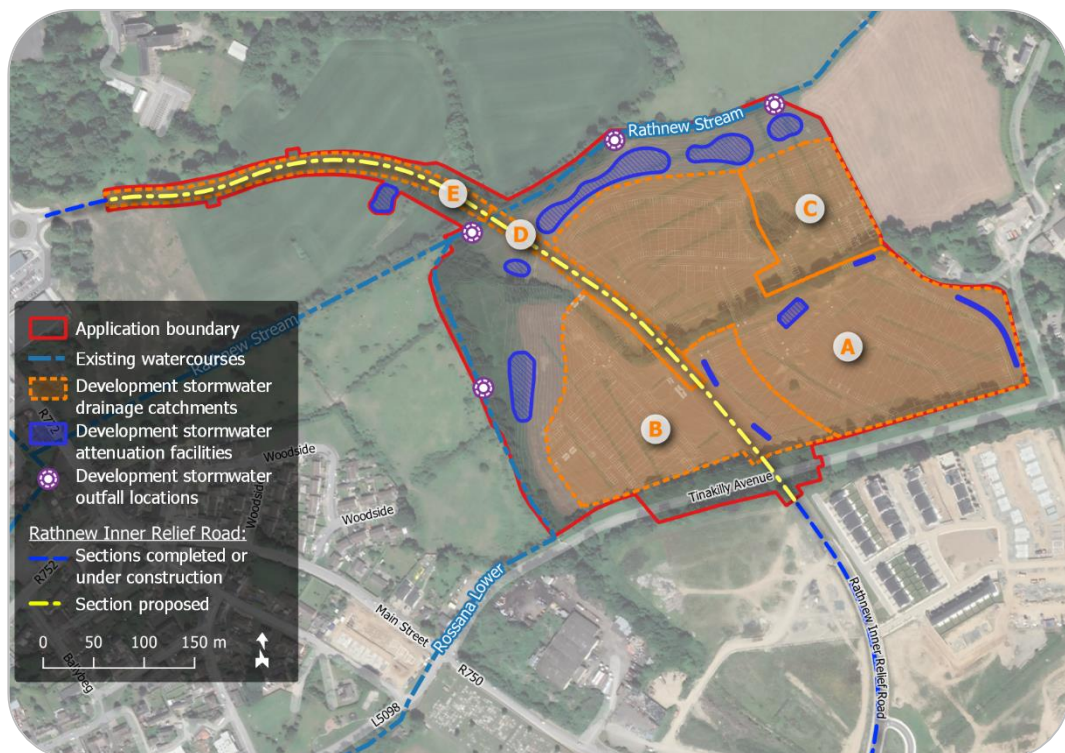
Figure 3 – Proposed stormwater drainage arrangements (map data and imagery: EPA, OSM Contributors, Google)
